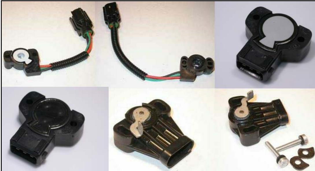
Row 1: LH blade, RH blade, D drive LH, Row 2: D Drive RH, Kinsler AC, Kinsler CW
