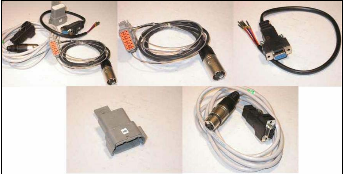
Row 1: CIM assembly, CIM car cable, CIM D9 loom, Row 2: CIM module, CIM pc cable
