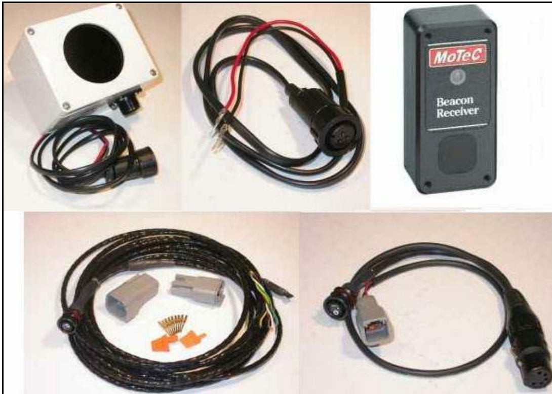
Row 1: BTX transmitter kit, BTX loom, BR2 beacon receiver, Row 2: BR2 loom, BR2 Comms loom
